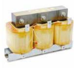
Blocking reactors, together with capacitor banks, create power factor correction and harmonic current filtering banks. This type of reactor is usually constructed with a magnetic core that can guarantee high linearity values even with large increases in current compared to the nominal value. A detuning power factor correction system prevents any amplification of harmonic currents and voltages caused by resonance between the capacitor and inductance capacitance of the electrical system.
